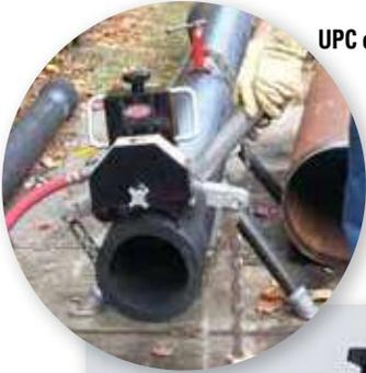
UPC636A on ductile iron
