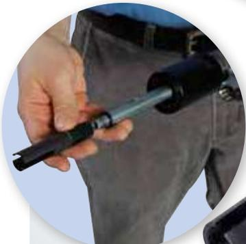
FTP2000UNIV & PL688 attaching to coupling nut
