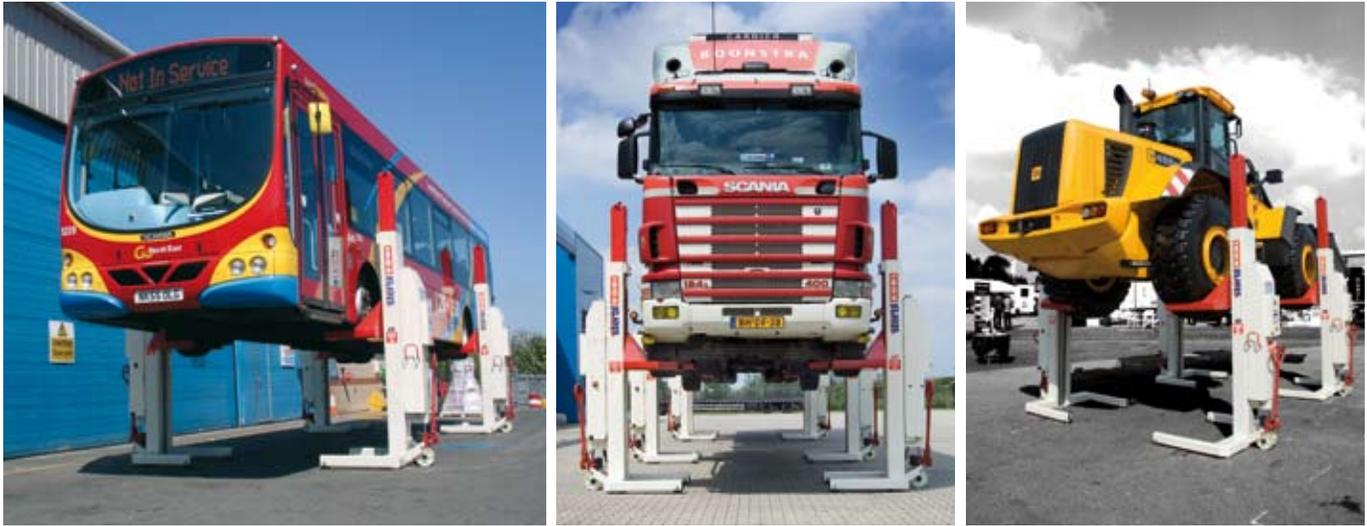
Wireless mobile column lifts are available in the following capacities per column:
