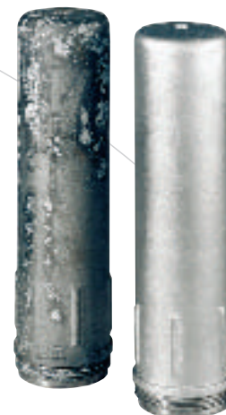
Untreated and Alu-chromed filter bowls after a salt spray test to DIN 50021 SS > 250 hours
