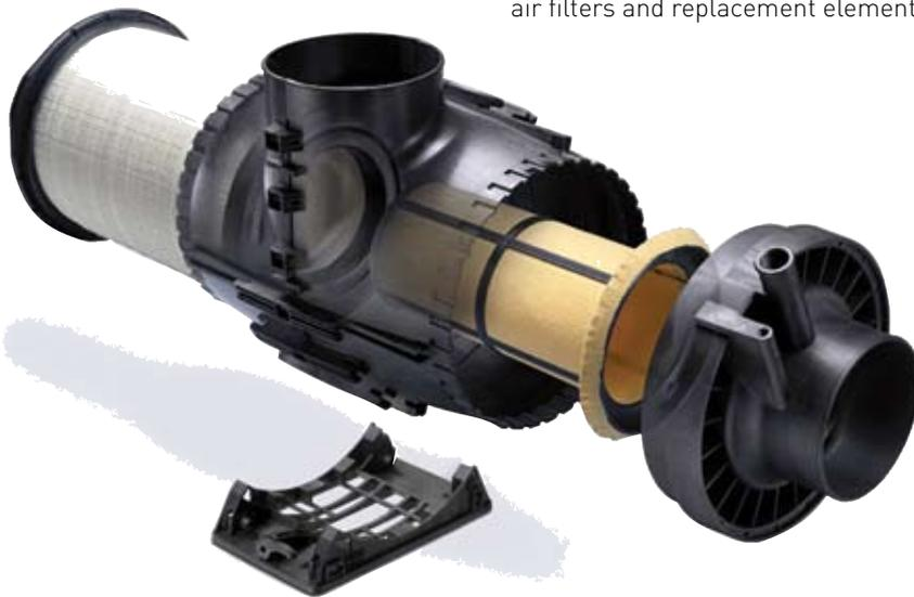
**The ECO III** is Racor's newest engine air filter, designed specifically to be the most versatile filter on the market, allowing for multiple inlet/outlet angle positions, left or right hand element removal and outlet configurations, with CCV and gauge connections built in. Designed for 250-500HP engines the ECO III's versatility makes it ideally suited for truck, bus and coach applications.
